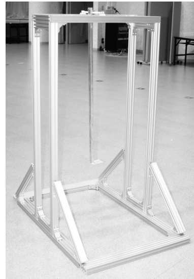
図10 慣性モーメント計測治具 Fig.10 Moment of inertia measurement device
